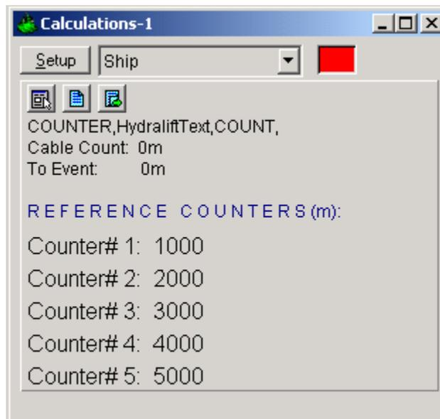
Once the Calculations window has been opened and configured, the five reference counters can be modified using the Reference Counters page of the Configure Counter dialog. (Note: the Configure Counter dialog can be directly accessed from the Calculations window by clicking the
