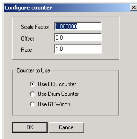
If you determine that the incoming cable count is incorrect, possibly due to a miscalibration of the counter itself, a compensating Scale Factor can be entered here. This can also be used to convert incoming units to the desired units if necessary. Also an offset value and cable payout rate factor can be entered in the appropriate dialogs. The
