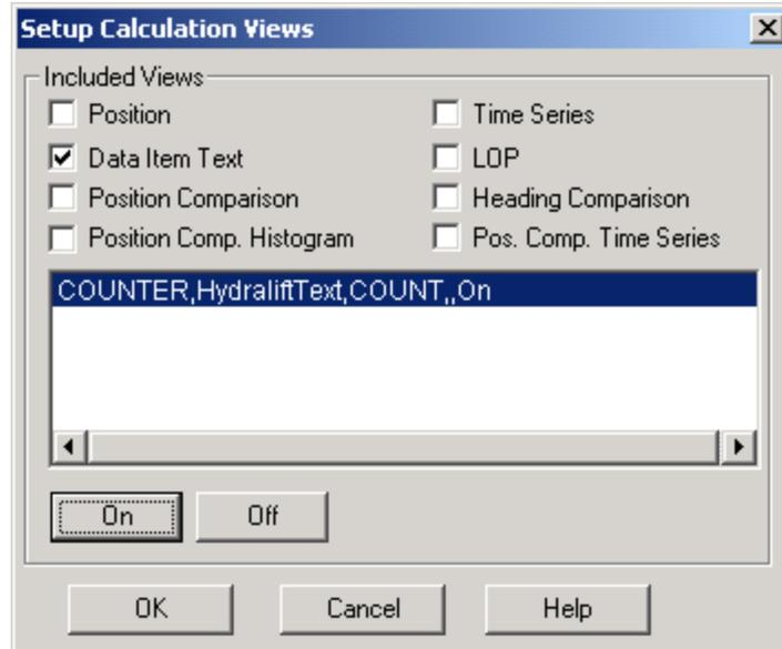
3. In the Setup Calculation Views dialog box select the Data Item Text checkbox. Then turn On the COUNT data item by selecting the COUNT data item from the list and click the On button.
